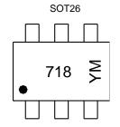
718 = Product Type Marking Code YM = Date Code Marking Y or  $\overline{Y}$  = Year (ex: C = 2015) M or  $\overline{M}$  = Month (ex: 9 = September)
