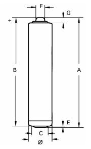
Type Designation 4906 **Designation IEC** LR6 Zn-MnO<sub>2</sub> (Alkaline) System Shelf Life (Coding)\* 5 years Nominal Voltage [V] 1.5 Typical Capacity C [mAh]  $2850 \ ({\it discharge with high-resistance})$ Permissible Temperature Range - 10 °C ... 50 °C Weight, approx. [g] 24 7.62 Volume [ccm] Dimensions [mm] min: max: Ø A B C E 14.5 13.5 50.5 49.5 7.0 0.5 5.5
