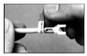
Pick up tab to remove marker from book. Complete the wrap, and flip the tab off.
