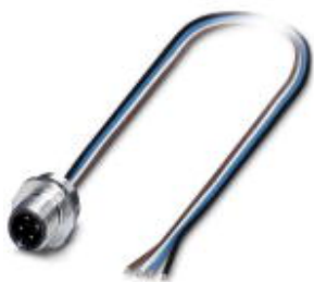
Sensor/actuator flush-type plug, 4-pos., stainless steel, A-coded, front/screw mounting with M16 thread, with 0.5 m TPE litz wire, 4 x 0.34 mm 2
