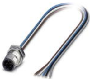
Sensor/actuator flush-type plug, 5-pos., M12 SPEEDCON, B-coded, rear/screw mounting with M12 thread, with 0.5 m TPE litz wire, 5 x 0.34 mm 2
