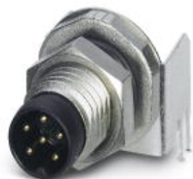
Sensor/actuator flush-type connector, plug, 6-pos., M8, rear/screw mounting with M8 fastening thread, with angled solder connection
