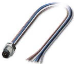
Sensor/actuator flush-type plug, 6-pos., M8, rear/screw mounting, with M8 thread, with 0.5 m TPE litz wire, 6 x 0.14 mm 2
