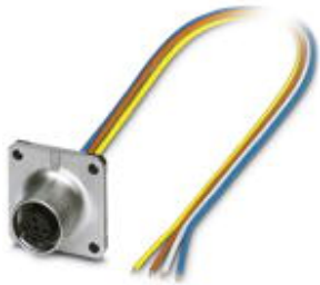
Sensor/actuator flush-type socket, 4-pos., M12, D-coded, front/square flange mounting, with 0.5 m TPE litz wire, 4 x 0.34 mm 2
