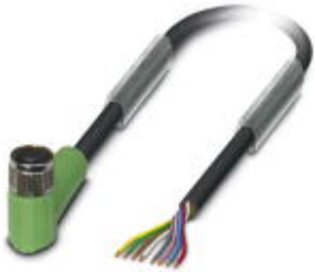
Sensor/Actuator cable, 8-position, PUR halogen-free, black RAL 9005, free cable end, on Socket angled M8, Cable length: 3 m
