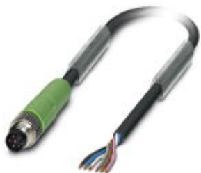
Sensor/Actuator cable, 6-position, PUR halogen-free, black-gray RAL 7021, Plug straight M8, on free cable end, Cable length: 10 m
