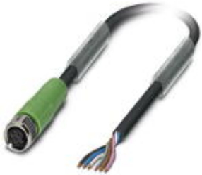
Sensor/Actuator cable, 6-position, PUR halogen-free, black-gray RAL 7021, free cable end, on Socket straight M8, Cable length: 10 m
