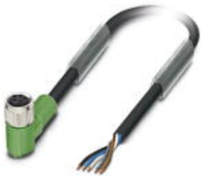
Sensor/Actuator cable, 5-position, PUR, black-gray RAL 7021, free cable end, on Socket angled M8, B-coded, Cable length: 10 m
