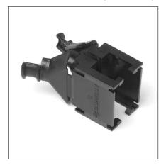
Separate strain relief hoods are available for all standard plugs SMS—P1. The hoods consist of identical halves that snap into position on the plug and are secured in place with the cable tie drawn tightly around the cabe entry collar. Catalog numbers designate a complete hood (2 halves) SMS—H1 The cable tie is not included (TF4D – TF5D) Two three and four position hoods are single piece units
