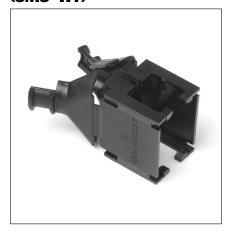
Separate strain relief hoods are available for all standard plugs SMS—P1. The hoods consist of identical halves that snap into position on the plug and are secured in place with the cable tie drawn tightly around the cabe entry collar. Catalog numbers designate a complete hood (2 halves) SMS—H1 The cable tie is not included (TF4D – TF5D)
