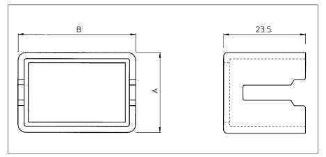
When pins are inserted into the panelmount receptacle half (SMS–R1) of the QIKMATE connector, an optional pin protection shroud can be installed.
