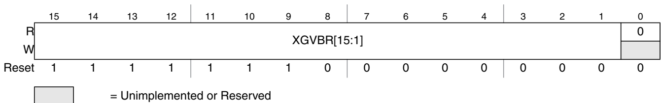
Figure 10-9. XGATE Vector Base Address Register (XGVBR)
