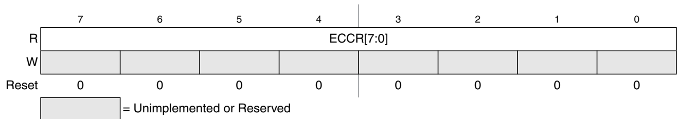
Figure 28-21. Flash ECC Error Results Low Register (FECCRLO)
