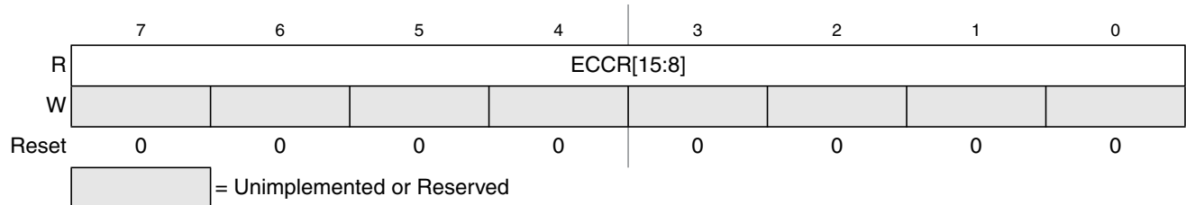
Figure 24-20. Flash ECC Error Results High Register (FECCRHI)
