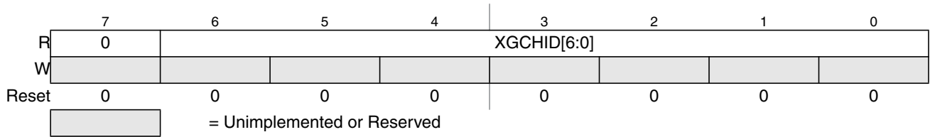
Figure 10-4. XGATE Channel ID Register (XGCHID)
