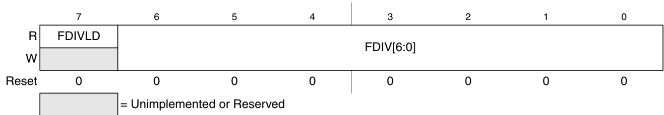
Figure 29-5. Flash Clock Divider Register (FCLKDIV)
