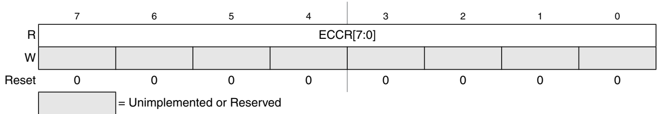
Figure 29-21. Flash ECC Error Results Low Register (FECCRLO)
