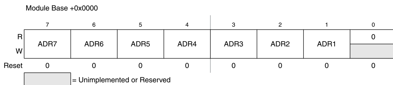
Figure 15-3. IIC Bus Address Register (IBAD)
