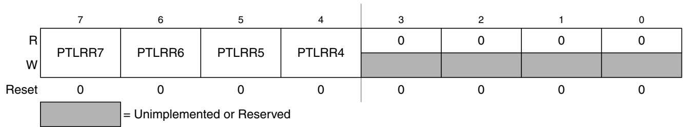
Figure 2-98. Port L Routing Register (PTLRR)
