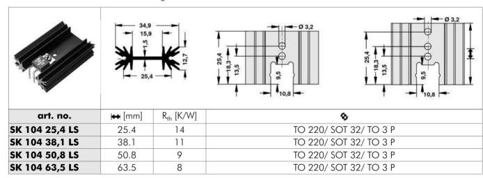
special lengths and transistor drillings on request
