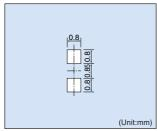
The recommended thickness of the screen mask for soldering is between 100 and 150µm. The hole size of the screen mask should be same as the recommended land pattern or smaller.
