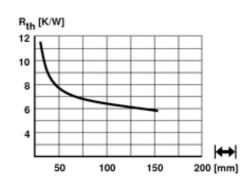
33 x 10 mm, for pcb mounting SK 400 ... x M3 L
