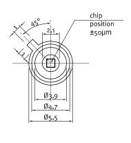
UVA-only SiC based UV photodiode A = 1,0 mm<sup>2</sup>
