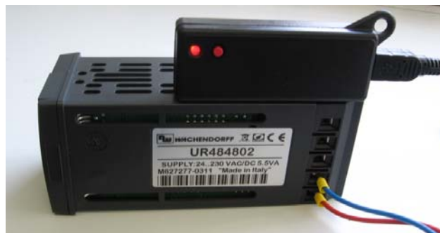
Figure 3: Inserting Programming module on UR4848xx
