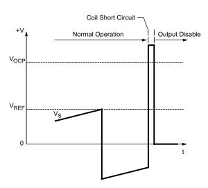
Figure 4. Motor coil short circuit protect circuit operation. Overcurrent that flows without passing the sense resistor is undetectable. To recover the circuit after protection operates, VDD must be cycled and started up again.
