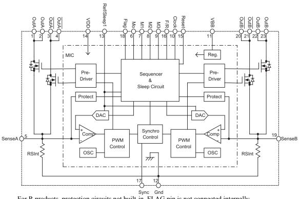
For R products, protection circuits not built-in. FLAG pin is not connected internally.
