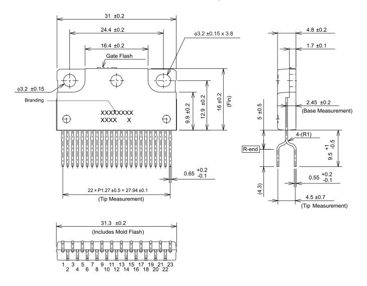
Terminal core material: Cu Terminal treatment: Ni plating and solder dip Leadform: 2151
