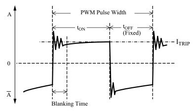
Figure 2. SENSEx pins pattern during PWM control
