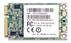
When operating on channels in the UNII-2 and UNII-2 Extended bands that are in the 5GHz portion of the frequency spectrum and are subject to Dynamic Frequency Selection requirements, the SDC-PE15N fully conforms to applicable regulatory requirements. In the event that specified types of radar are detected by the network infrastructure, the SDC-PE15N fully conforms to commands from the infrastructure for radar avoidance.
