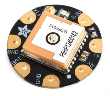
This module is the best way to add a GPS to your wearable project. It's part of the Adafruit Flora series of wearable electronics, designed specifically for use with the Flora motherboard. Installed on the PCB is the latest of our Ultimate GPS modules, a small, super-thin, low power GPS module with built in data-logging capability! This module's easy to use, but extremely powerful:
