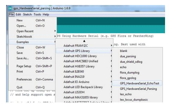
Wire up the GPS module according to the hookup. Check your board and serial port settings (https://adafru.it/aRS) and upload this sketch to your Flora using the Upload button in the IDE. Open up the **Serial Monitor**.
