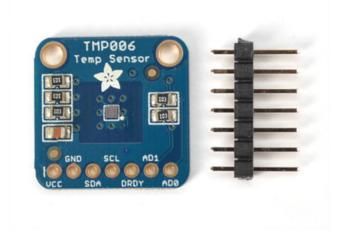
Unlike most temperature sensors, the TMP006 does not require contact with the object it is measuring. It uses a very sensitive thermopile to measure the infrared energy being emitted from the surface of the object.
