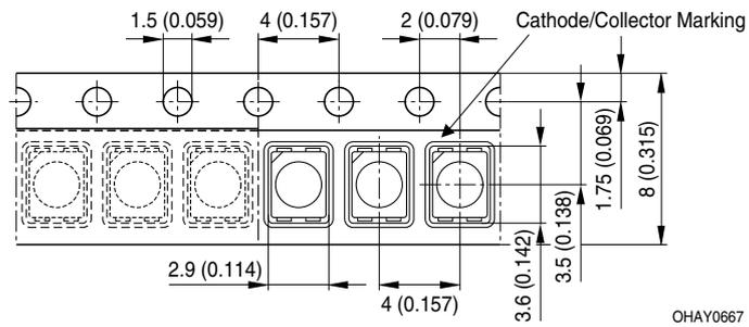
**Tape and Reel****Gurtverpackung**8 mm tape with 2000 pcs. on  $\varnothing$  180 mm reel, 8000 pcs. on  $\varnothing$  330 mm reel
