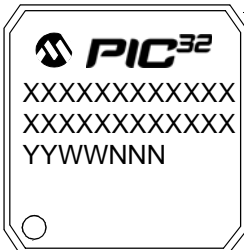
100-Lead TQFP (12x12x1 mm)
