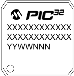
100-Lead TQFP (14x14x1 mm)
