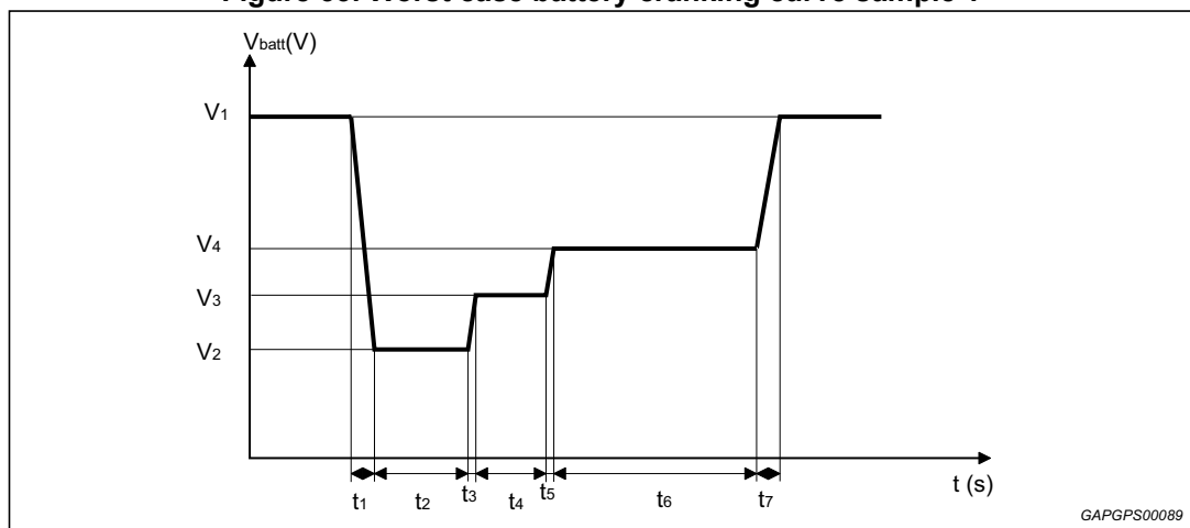
Figure 33. Worst case battery cranking curve sample 1
