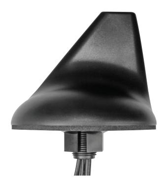
Pulse is proud to introduce a new state-of-the-art direct mount multi band antenna. This body mount antenna operates from 698 thru 5875 MHz, including LTE. The antenna is ideal for voice, mobile data, Public Safety, WLAN and asset tracking applications. The rugged, yet aesthetically pleasing design provides UV and IP-65 protection to ensure a long, reliable, maintenance-free life
