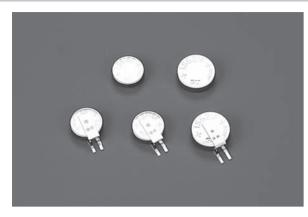
TS lithium rechargeable batteries are high capacity 1.5V type non-reflowable rechargeable batteries that provide sufficient discharge capacity with a charge voltage of less than 2.0V, and are intended for support of recent low-operating-voltage mobile devices.
