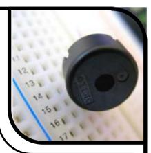
We will once again rely on its incredible speed which will let it mimic analog behavior. To do this, we will attach a piezo element to one of the Arduino's digital pins. A piezo element makes a clicking sound each time it is pulsed with current. If we pulse it at the right frequency (for example 440 times a second to make the note middle A) these clicks will run together to produce notes. Let's get to experimenting with it and get your Arduino playing "Twinkle Twinkle Little Star".
