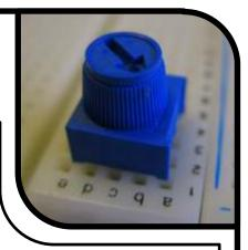
it to a digital number between 0 (0 volts) and 1023 (5 volts) (10 bits of resolution). A very useful device that exploits these inputs is a potentiometer (also called a variable resistor). When it is connected with 5 volts across its outer pins the middle pin will read some value between 0 and 5 volts dependent on the angle to which it is turned (ie. 2.5 volts in the middle). We can then use the returned values as a variable in our program.
