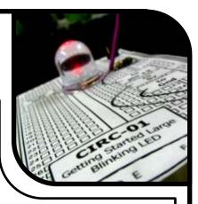
everything in. Once the circuit is assembled you'll need to upload the program. To do this plug the Arduino board into your USB port. Then select the proper port in Tools > Serial Port > (the comm port of your Arduino). Next upload the program by going to File > Upload (ctrl+U). Finally, bask in the glory and possibility that controlling lights offers.
