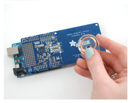
Using the Adafruit NFC Shield with I2C
