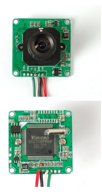
If you'd like to get NTSC video out to connect to a TV or monitor, solder another black wire to the second Ground pin, and a yellow wire to the CVBS pin.
