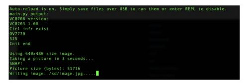
Be aware saving the image to the card takes some time as the data is transferred over both a serial connection from the camera and the SPI connection to the micro SD card. A full image capture at 640x480 pixels takes about 30 seconds, but might take longer depending on your board and micro SD card speed.
