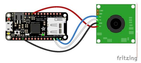
Just like connecting the camera to an Arduino you need to connect these wires:
