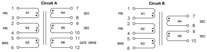
Primary windings (N1 and N2) and Secondary windings (N4 and N5) must be connected in parallel on the customer PCB.
