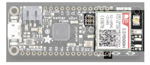
Now to the fun part, the cellular module. There's a few pins that are used to control the module. It uses SoftwareSerial to communicate with the microcoller
