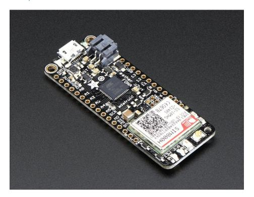
At the Feather 32u4's heart is at ATmega32u4 clocked at 8 MHz and at 3.3V logic, a chip setup we've had tons of experience with as it's the same as the Flora (https://adafru.it/dVl). This chip has 32K of flash and 2K of RAM, with built in USB so not only does it have a USB-to-Serial program & debug capability built in with no need for an FTDI-like chip, it can also act like a mouse, keyboard, USB MIDI device, etc.
