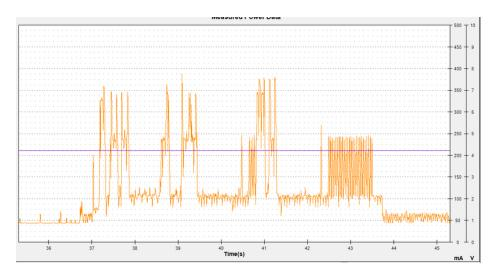
Sending an MQTT packet (about 200 bytes)
