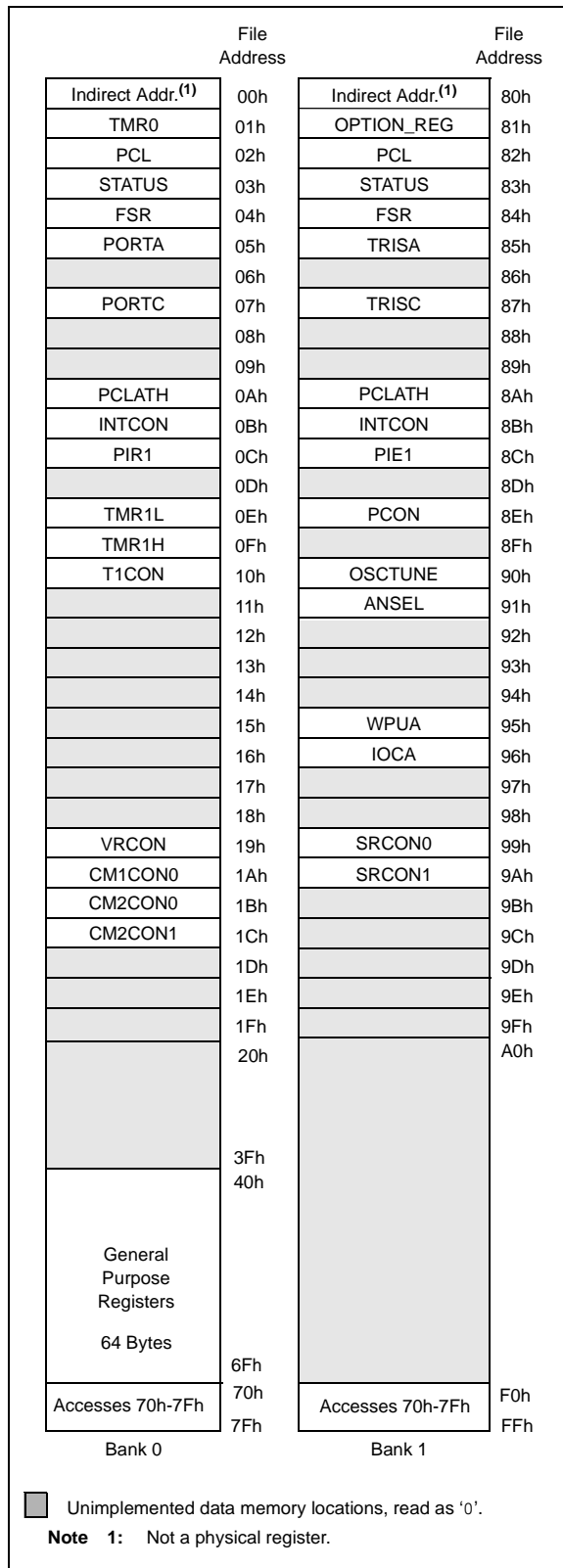
FIGURE 2-3: DATA MEMORY MAP OF THE PIC16F610/16HV610
