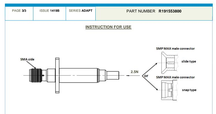
1. Connect the SMA side of the adapter with the measurement test equipment.
