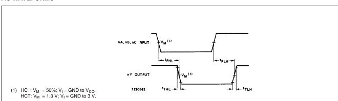
Fig.6 Waveforms showing the input (nA, nB, nC) to output (nY) propagation delays and the output transition times.
