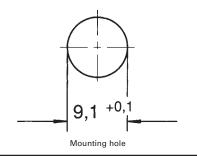
Accessories Signal lamps with integrated LED - 9.1 mm
