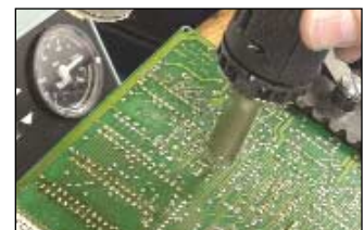
Through hole rework with the DSV80
