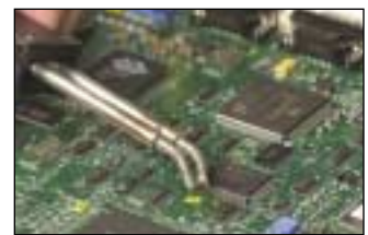
The WTA50 is perfect for removing Melf's from a SMT board.
