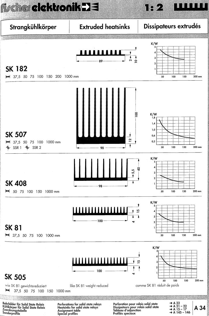
Heatsinks for solid state relays Assignment table Special profiles
