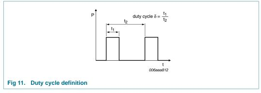
The current ratings for the typical waveforms as shown in Figure 8, 9 and 10 are calculated according to the equations:  $I_{F(AV)} = I_M \times \delta$  with  $I_M$  defined as peak current,
