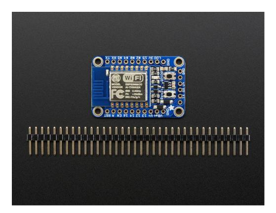
Each order comes with one assembled and tested HUZZAH ESP8266 breakout board, and a stick of 0.1" header that you can solder on and plug the breakout into a breadboard. A soldering iron and solder is required for that, and aren't included. You'll also need a USB-serial cable such as a USB console cable (Windows only) (https://adafru.it/dDd), FTDI Friend (any OS) (http://adafru.it/284), or FTDI cable (any OS) (http://adafru.it/70)to upload software to the HUZZAH ESP8266!
