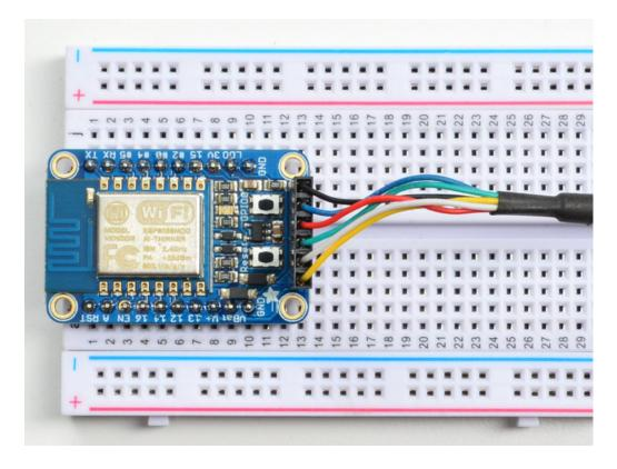
If using a console cable, connect the black wire to ground, red wire to V+, white wire to TX and green wire to RX
