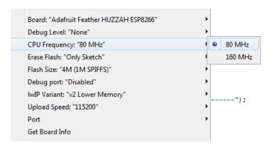
115200 baud upload speed is a good place to start - later on you can try higher speeds but 115200 is a good safe place to start. You can move down to lower speeds if you are having upload issues, or speed it up if your setup is stable, for faster uploads!
