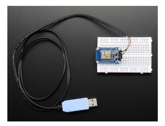
Each module comes pre-loaded with NodeMCU's Lua interpreter (NodeMCU 0.9.5 build 20150318 / Lua 5.1.4 to be specific) (https://adafru.it/inA), you can run commands, and 'save' Lua programs directly to the module's Flash using a USB-Serial converter cable.
