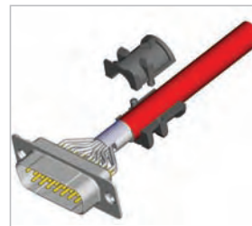
Attach the strain relief around the cable
