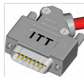
Assemble the other half (screwing force: 100-120 Ncm)
