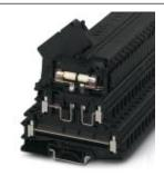
Fuse modular terminal block, Connection method: Screw connection, Cross section: 0.2 mm<sup>2</sup>- 4 mm<sup>2</sup>, AWG: 24 - 12, Nominal current: 32 A, Nominal voltage: 400 V, Width: 8.2 mm, Fuse type: G / 6,3 x 32, Fuse type: Glass, Mounting type: NS 35/7,5, NS 35/15, NS 32, Color: black
