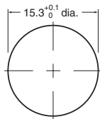
Panel Cutout Dimension Panel thickness = 1 to 4 mm
