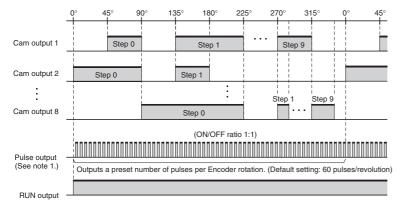
Note 1: The number of pulses per Encoder rotation and the pulse output start angle can be set.
