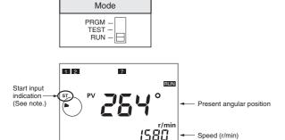
Note: For 16/32-output models, be sure that the start input is ON and that the start input indicator is lit. Outputs (including the cam, pulse, and run outputs) will not function if the start input is OFF. The 8-output models do not have a start input.
