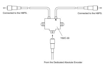
Use the cable marked with a triangle when connecting only one H8PS Cam Positioner to the Parallel Input Adapter.
