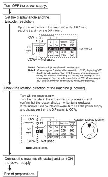
Note: Changes to DIP switch settings are enabled when the power is turned ON.
