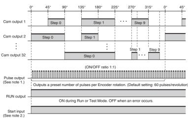
Note 1: The number of pulses per Encoder rotation and the pulse output start angle can be set.
