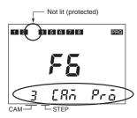
Set the cam number to be protected (and not displayed) to 3 with the CAM Keys = and then press the WRITE Key. The output display will go out.
