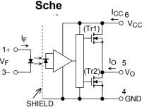
A  $0.1\mathchar`-\mu F$  bypass capacitor must be connected between pins 6 and 4. (See Note 6.)
