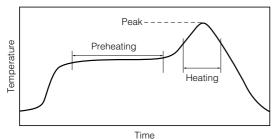
For soldering (Example : Sn/Pb)
