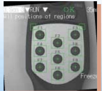
Gray Search Processing of multiple inspection areas with position compensation enabled – 35ms
